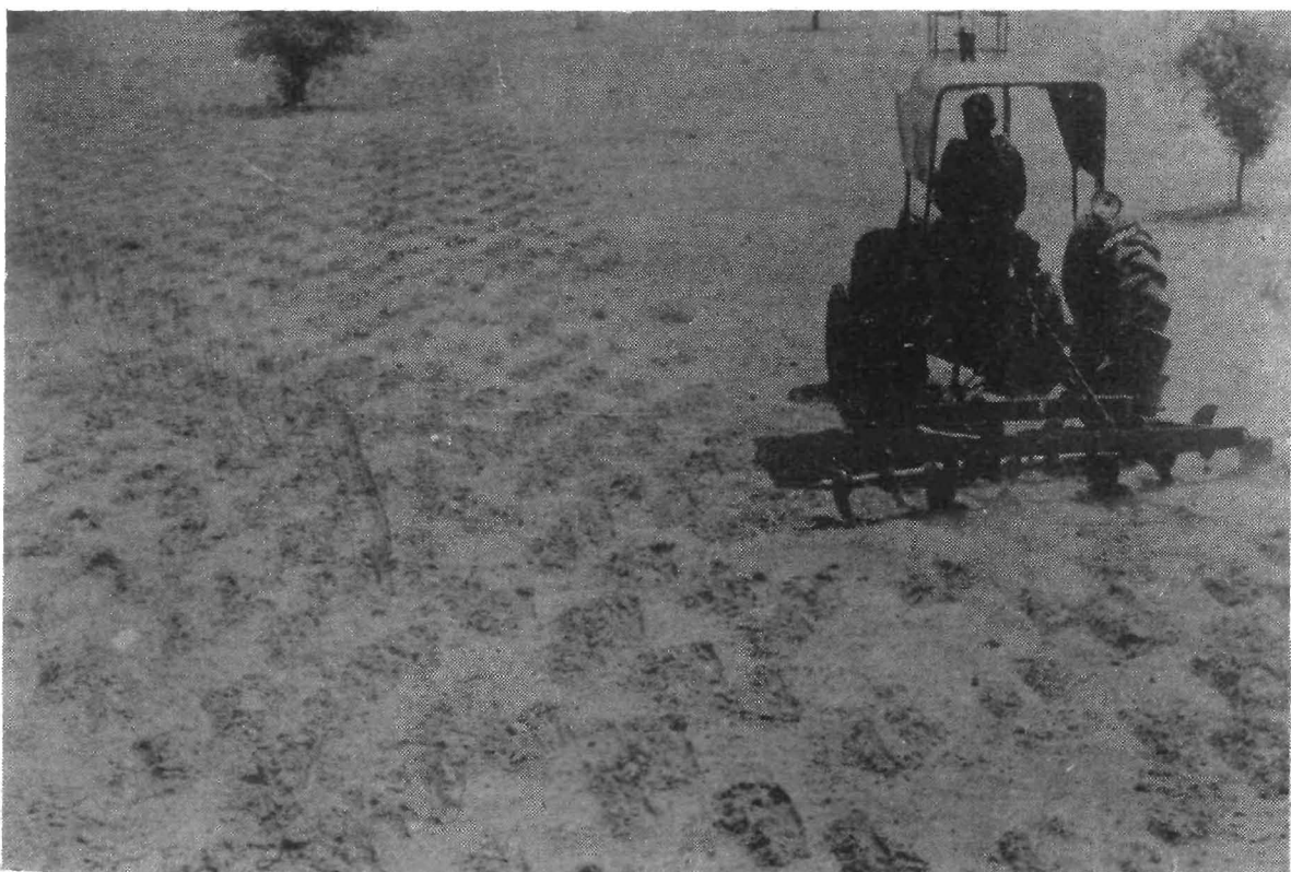
CAZRI Pitting Disk— a device for micro pits for water conservation
