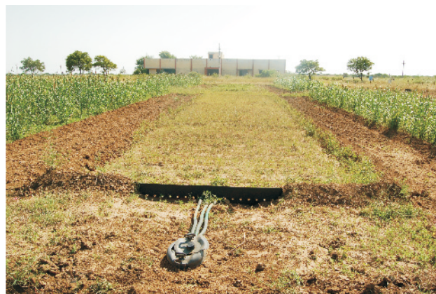
Fig. 7. Field views of (a) sorghum-clusterbean intercropping and (b) unploughed fallow plot with multi-slot divisor and runoff collection tank (Year 2013)
